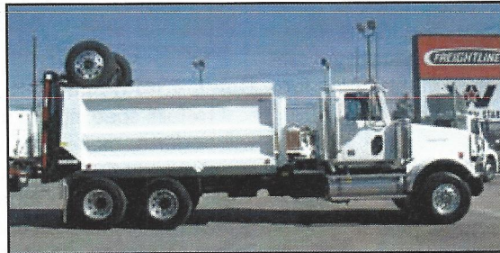
This 10-wheel dump truck has an airlift "Booster" axle, shown in the raised position.
