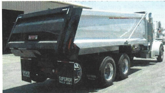
This 10-wheel dump truck has an airlift "Pusher" axle, shown in the raised position.
