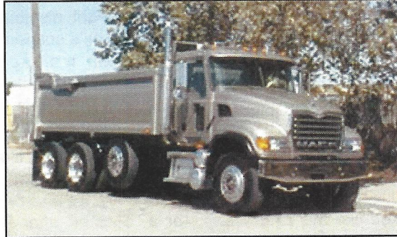
This 10-wheel dump truck has an airlift "Pusher" axle, shown in the raised position.
